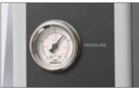
Gauge to display the pressure of the upper roller
